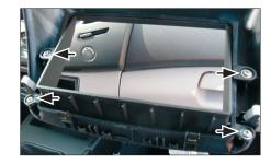
4. Mount facia plate to OEM-Panel (with original screws)
