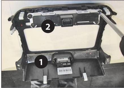
9. Remove hazard light switch (1) from OEM head unit - attach it to double DIN facia plate
