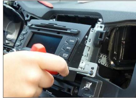
6. Remove screws of OEM head unit
