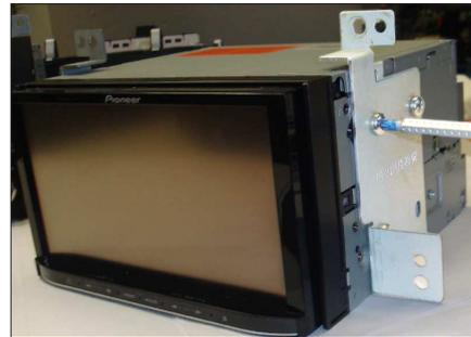
7. Attach metal mounting brackets to Pioneer Navigation
